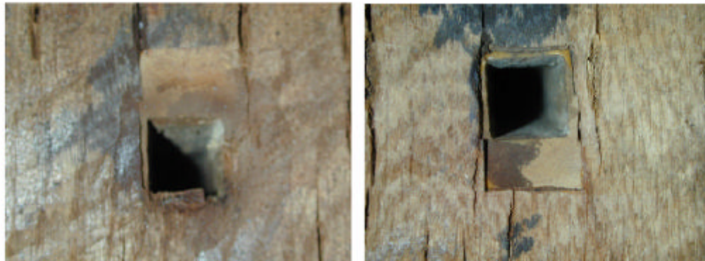
Figure 8 – Spike holes from yellow ES-30 (field left, gauge right) after 1,000,000 cycles..
