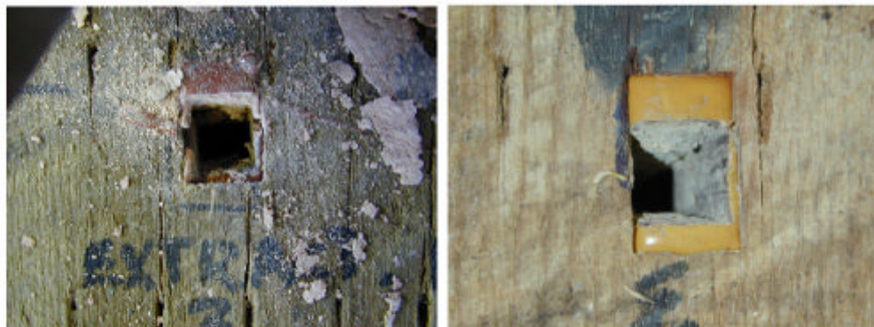
Figure 6 – Example of spike holes after 10 extraction cycles showing red ES-25 (left) and yellow ES-50 (right). Same flaking occurred in both materials during extraction (yellow ES-50 right, cleaned before photo was taken). Note slight depression around yellow material also.
