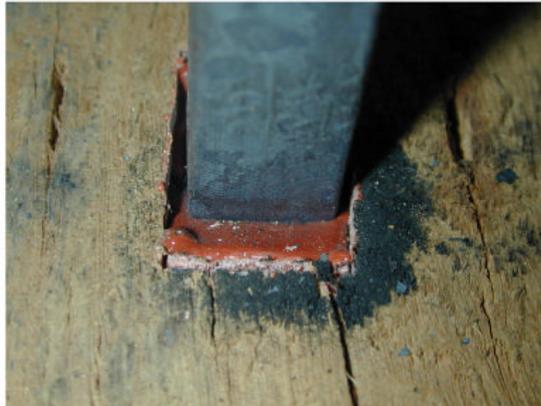
Figure 5 – Start of insert/extract tests. Note filler plug pressed into the hole.
