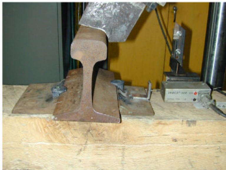
Figure 2 – Close-up showing one end of setup with plate bracket and LVDT transducer visible.
