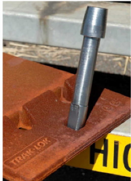
Acceptable lockspike hole
