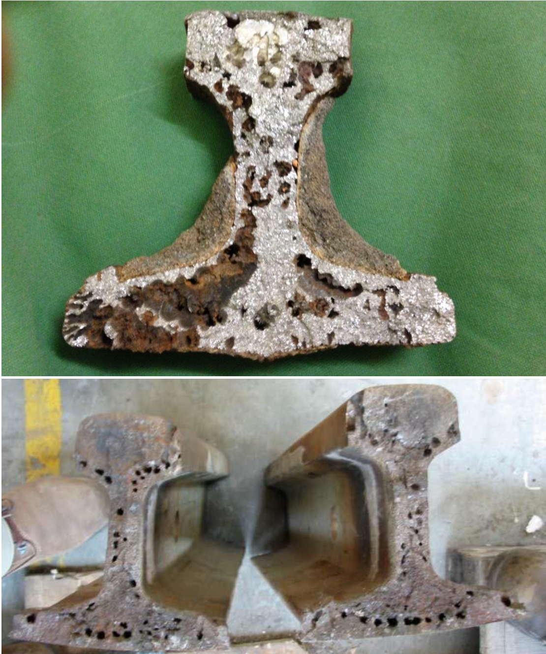
Figure 25: Rail Weld Defect (Porosity)
