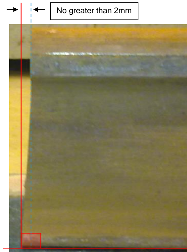
Figure 1: Rail end squareness vertical tolerance should be measured at 90° to the rail foot or head dependant on the angle of the cut and should be no greater than 2mm.
