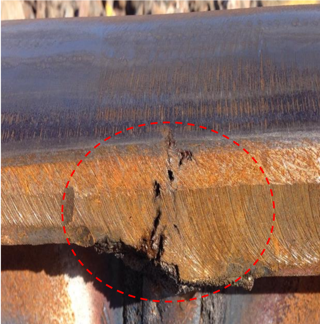
Figure 26: Rail Weld Defect (Surface breaking hot tear in weld)
