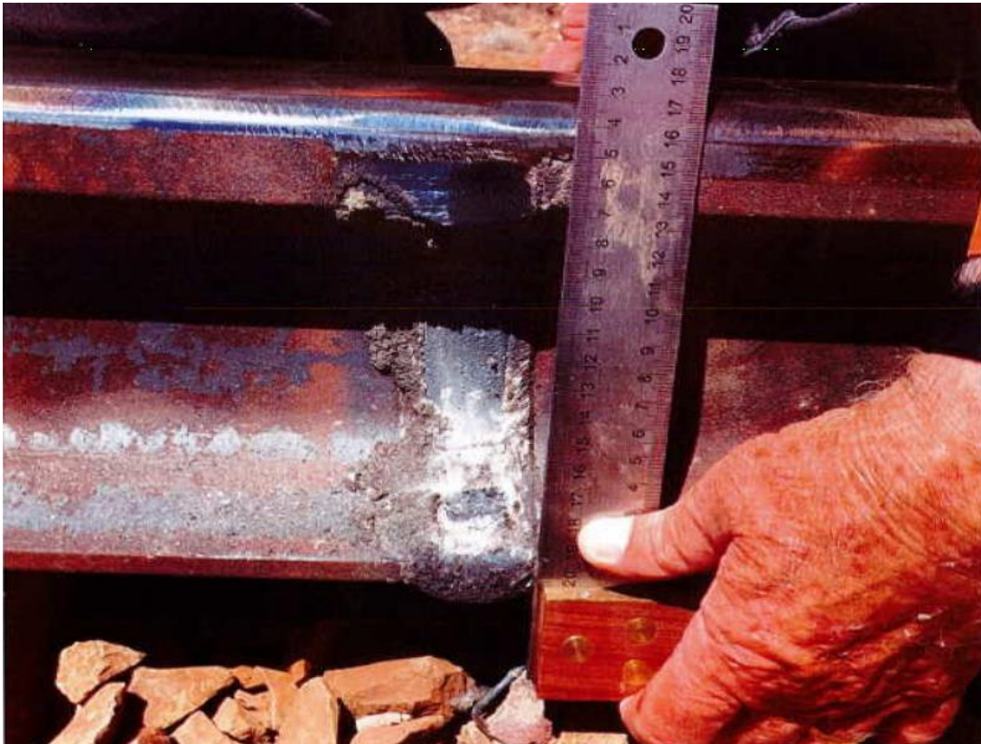
Figure 20: Poor vertical alignment of the weld collar measured with a square rule
