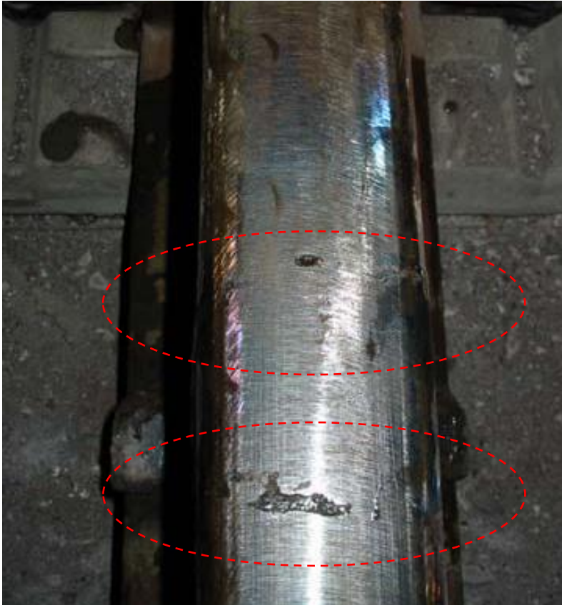
Figure 31: Rail Weld Defect (Sand Burns)
