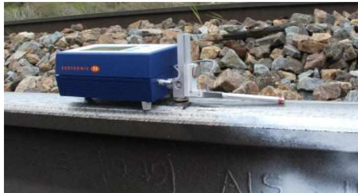
Figure 14: Measurement of Surface Roughness with a Typical Measuring System
