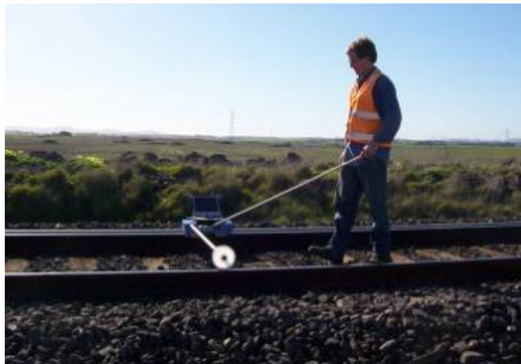
Figure 16: Measurement of Long Pitch Corrugations with a Typical Measuring System
