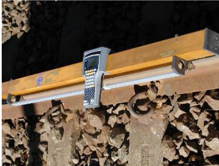
Figure 15: Measurement of Short Pitch Corrugations
