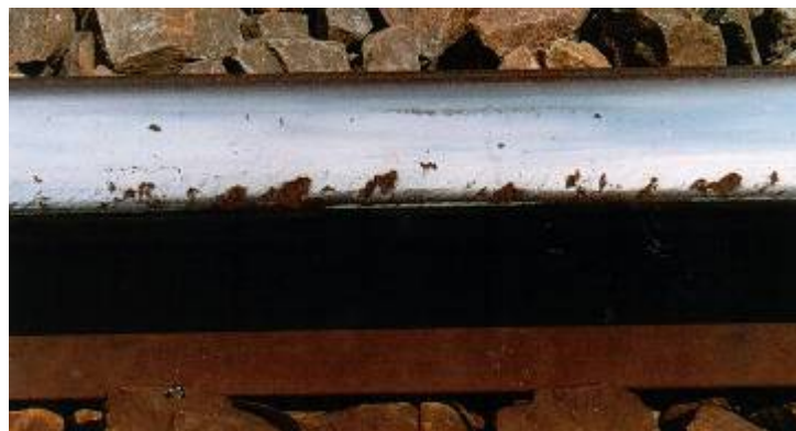
Figure 6: Example of Severe Gauge Corner RCF Defects on High Rails Requiring Application of the H3 Profile
