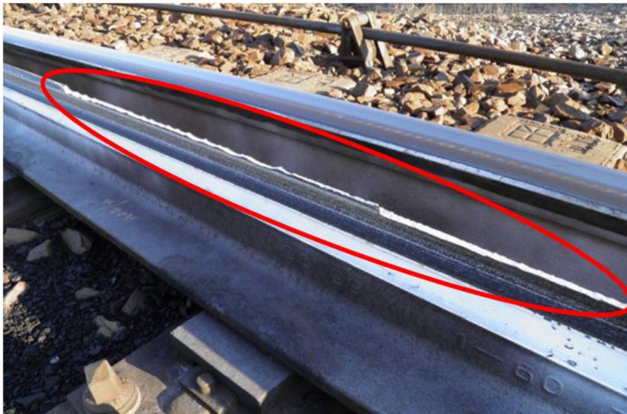
Figure 3-2: Switch blade with pieces broken away
