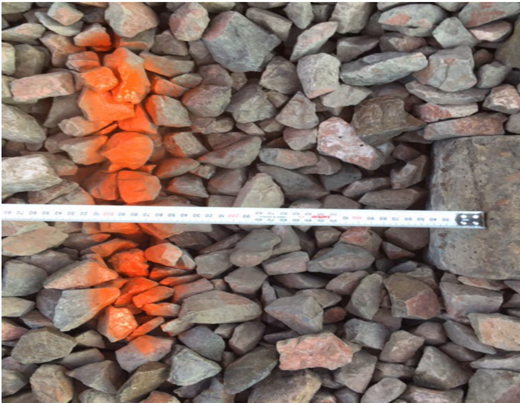
Figure C3 - The displacement at the end of the sleepers
