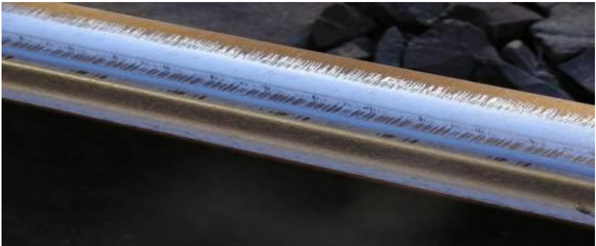
Figure 18 – Unacceptable severe profiling scratches
