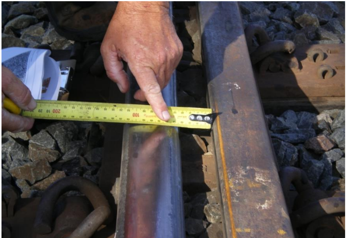
Figure 6-12 Measuring check rail flangeway width
