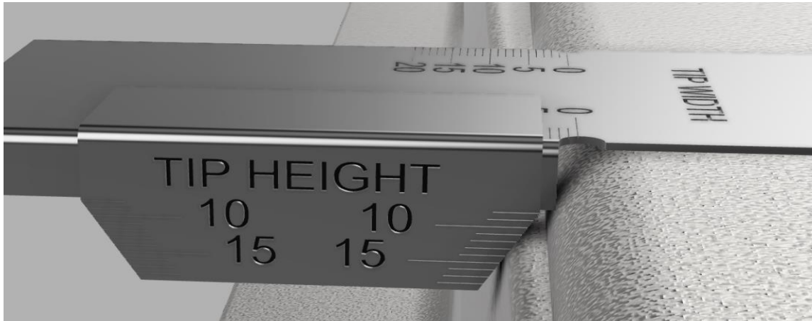
Figure 4-18 Switch tip width measurement when not using gauge.
