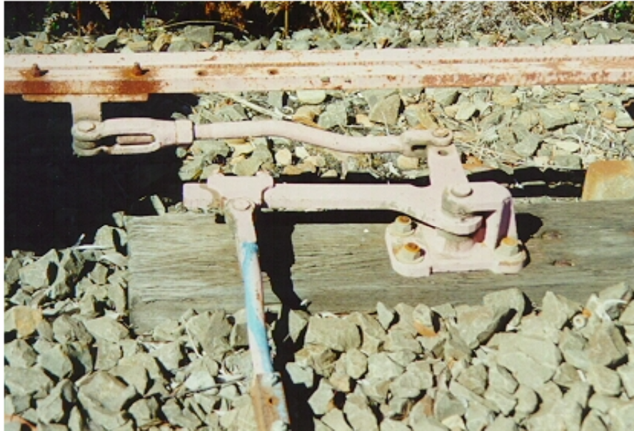
Figure 6.2.2 – Drop lug connection to channel rodding
