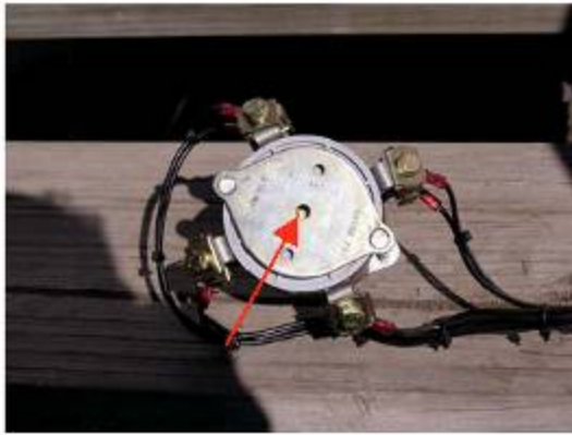
Rear of Santon switch showing spindle end not engaged in bearing plate.
