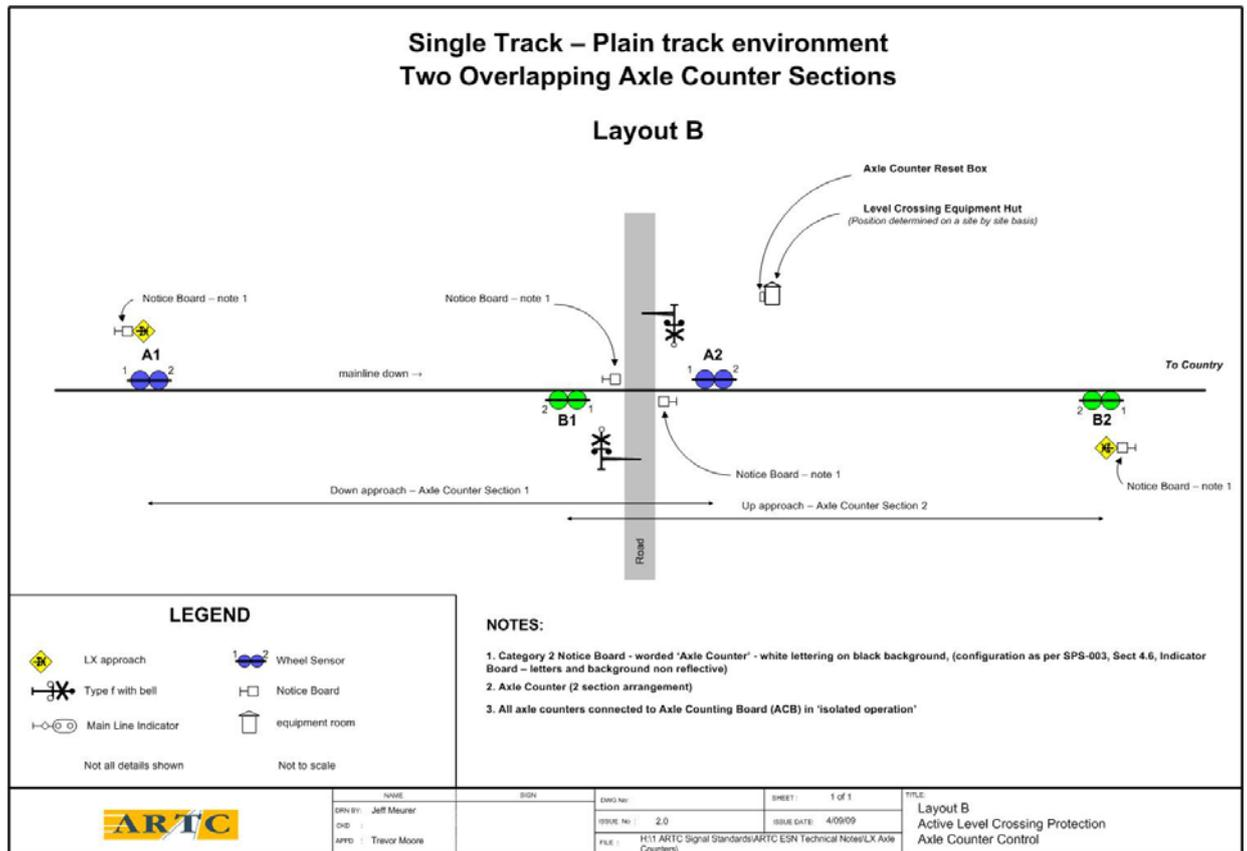
This arrangement may be used for an installation where hi-rail vehicles do not take on and take off. This is the simplest arrangement and with fewer components is less likely to result in technical miscount errors. This layout may be used only where layout A is not suitable.
