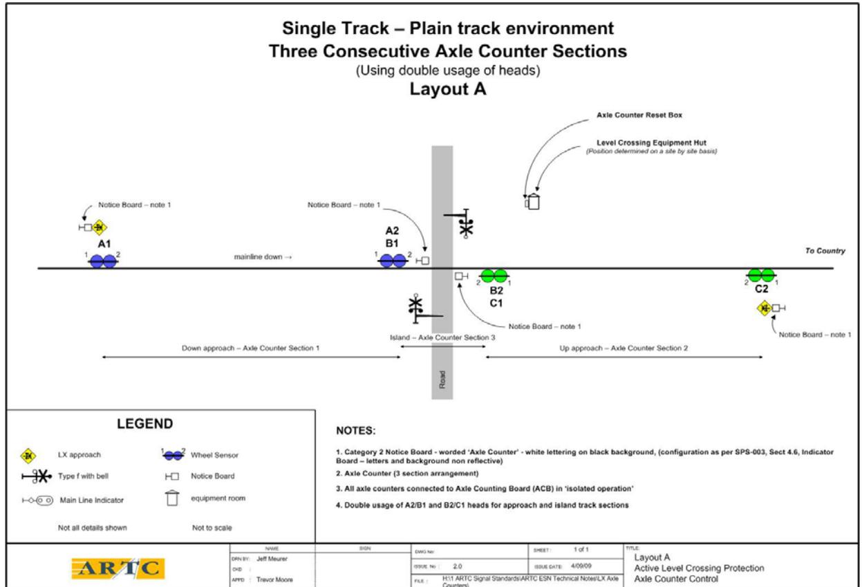
This arrangement is suitable for upgrading of a typical single line level crossing with 3 track circuits (i.e. Up approach, island and down approach tracks) as the three axle counters can readily substitute the existing track circuits. This is the preferred design configuration.
