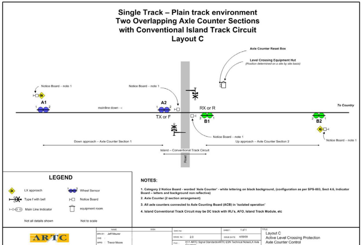
This arrangement is an improved arrangement over option A with regard to hi-rail operations i.e. hi-rail vehicles may enter or depart the crossing via the conventional island track circuit section. Independent axle counter track sections are used for the approaches. Island track protection is provided by a time delay (typically 8 seconds) on the axle counter section providing protection for the train passing over the crossing
