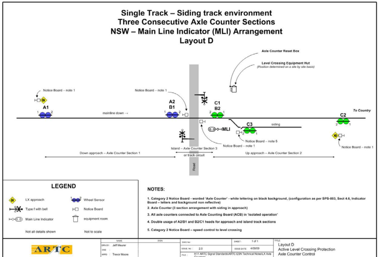
The approach requirements for all train paths to the level crossing shall be considered. Each approach path shall be recorded in the Level Crossing (Axle Counter) Control Table. Additional axle counters and or timing sections may be required to accommodate station stops or other regular train stopping locations.
