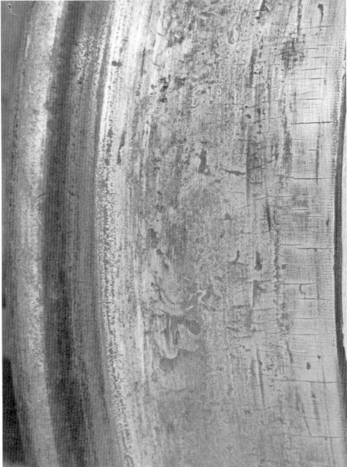
CLASS 4 THERMAL CRACK
