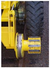
Friction drive hi-rail normally relies on the rubber road tyre to contact, drive and brake the rail wheel which is then in contact with the rail head. Once on track and with the rail wheels engaged, the plant is driven in the normal manner with the rubber road tyres rotating and providing motion to the rail wheels through friction. While the rubber road tyre provides drive to the rail wheels it is
