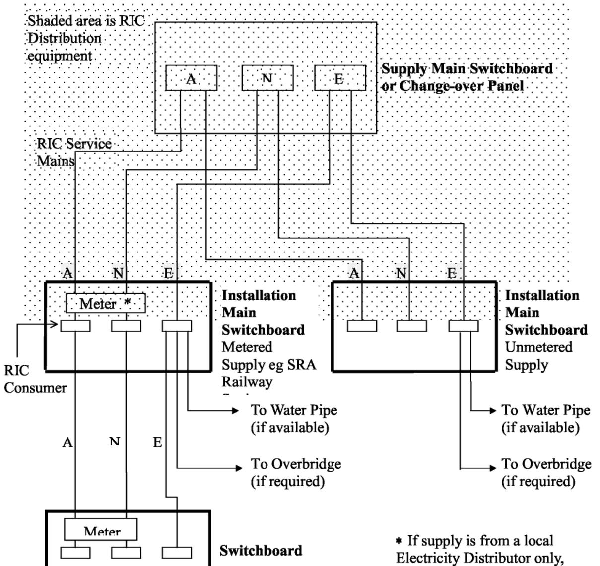
Figure 1 Connection of Installation Main Switchboards
