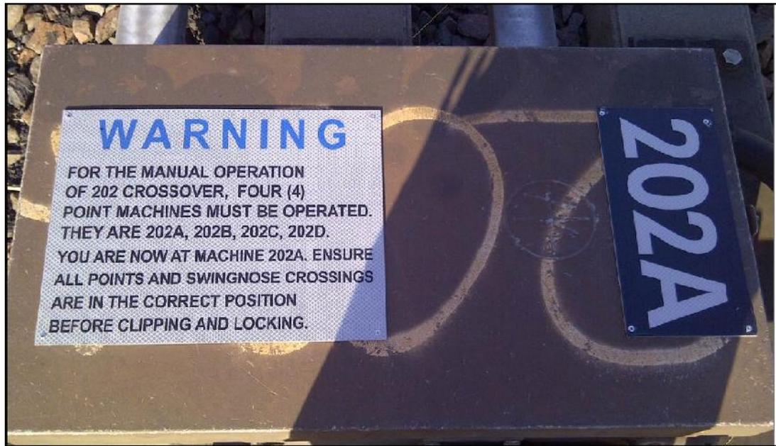
Figure D12 – Location of Points Manual Operation Warning Notice on D84M motor.
