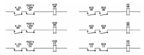
**RSR**: the A\_(ROUTE)\_RSR responds directly to the control system route request URR. The A\_(ROUTE)\_RSR bit is passed across the dual link, and received on the other side as B\_(ROUTE)\_RSR. The two are combined into the (ROUTE)\_RSR. This ensures that routes already set in the ONLINE master are correctly set in the other master if it has just rebooted.
