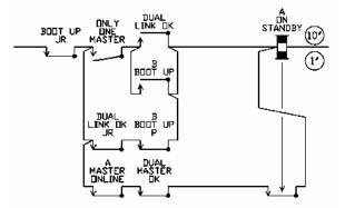
To maintain the quickest possible mastership change when the online master loses ON STANDBY, the indication bit sent to the control system takes BOOT UP JR in series with ON STANDBY.
