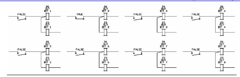
ASSIGN ~26\_IN\_BIT1 \* 26\_IN\_BIT2 \* ~26\_IN\_BIT3 \* ~26\_IN\_BIT4 \* ~26\_IN\_BIT5 \* ~26\_IN\_BIT6 \* ~26\_IN\_BIT7 \* ~26\_IN\_BIT8
