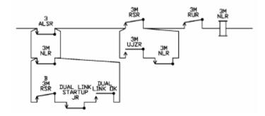
**Points NLR**, **RLR**: DUAL\_LINK\_OK + A\_MASTER\_ONLINE is included in series in the NLR and RLR logic to drop out these bits if the dual link fails and this master is not online. Combined with the DUAL\_LINK\_OK\_JR and the WLZSR, this allows the points lock relays to synchronise with the points detection when the master recovers from the dual link failure.
