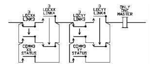
If the master is a split master arrangement, MP2 may still be communicating with the slaves but MP1 has shutdown. To provide ONLY\_ONE\_MASTER in this case, MP2 determines MP1 status on the basis of the Port 4 link to MP1. This status is sent to each slave, and is included in the link status bits each slave returns to both masters. The ONLY ONE MASTER logic for split masters is the same as that used by the non-split master.
