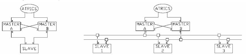
As shown in the diagrams, it may consist of a single slave in the same location as the masters, or several slaves in many locations. Where multiple slave locations exist, they are to be connected by fibre optic communications links utilising either Fibre Optic Modem Sets (FOMS), or where required according to section 2.6 of the specification "Design of Microlok Interlockings", a loop arrangement with Diversity Link Controllers (DLC).
