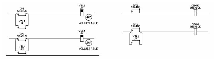
VSL1JR is used a common timer for both port 1 and port2 (the dual link). There is no delay in initialising the link to the slaves.
