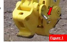
**Figure 2** shows a photo of a quick hitch safety pin (indicated by red arrow) used on the Yanmar excavators in the <u>engaged</u> position. (Some machines have different designs for quick hitch safety pins refer to the relevant operator manual for clarification)
