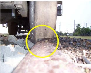
This photo clearly shows the dangers arising from not having the hi-rail guidance system recertified after having springs replaced. The hi-rail wheel has totally lost contact with the rail and would have certainly derailed had the problem not been spotted. Not all issues would be this obvious, with some wheels appearing to be on the rail, however the amount of down force on that wheel may have been severely compromised.
