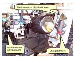
The portable hand pump shown here on the left is typical of the installation used on many of our existing vehicles. The pump must be manually connected to special fittings installed at the front & rear of the vehicle. If you have this type of system please ensure the pump is always in the vehicle.
